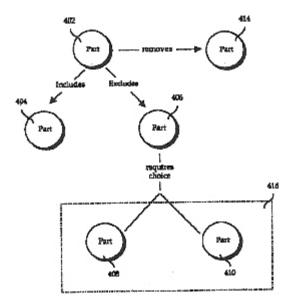
The dashed line box in Figure 4 is further described in the specification: "Parts 408 and 410 can be combined to form group 416. Group 416 can be defined by the user. If the user does not define group 416, the invention preferably creates group 416 to contain parts 408 and 410." '651 pat., col. 6, lns. 60-63.
