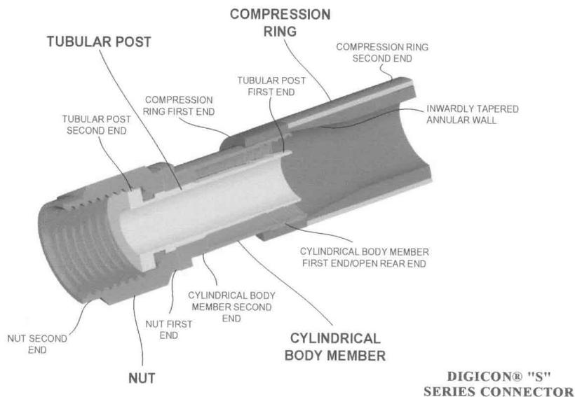
The nut rotatably engages the tubular post, the second end of the cylindrical sleeve engages the tubular post proximate the second end of the post and the compression ring has a non-tapered internal bore with a diameter commensurate with the first diameter of the outer wall
